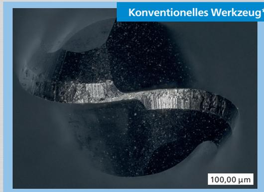
Wkz.-Ø 1 mm,  $n = 49300$  U/min ( $v_c, \max = 160$  m/min),  $v_f = 2465$  mm/min ( $f_z = 0.025$  mm/z),
